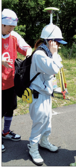
Fig. 1. A style of K-GPS measurement in this study. An antenna is mounted on a helmet.
