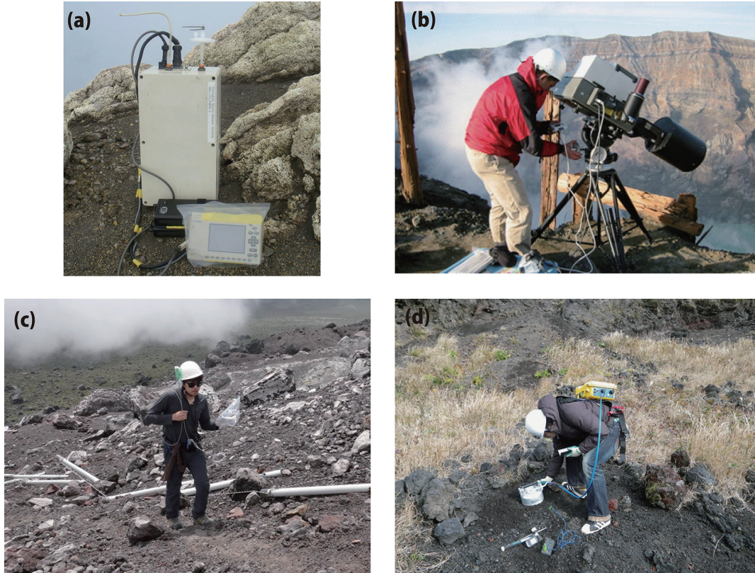
Fig. 1. Instruments and methods to measure volcanic gas. (a) Multi-GAS instrument. (b) Fourier transform infrared spectral radiometer (FTIR). (c) Walking traverse method using the DOAS technique (UV spectrometer USB2000+ based; OceanOptics, Inc.). (d) Closed Chamber Method (Portable Fluxmeter LICOR based; Westsystems, S. r. l.) for soil CO 2 flux measurement.
