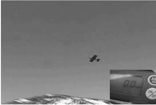
Fig. 8. A screenshot of the observation video on the H 2 S measurement mission. The main frame is an objective view of Sky-1 flight. Sub frame is the view of an onboard wireless video camera shooting the indicator of a portable H 2 S sensor. These two frame are synchronized by a video-editing software.
