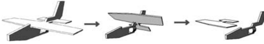
Fig. 2. Disassembling instructions for Sky-1. Sky-1 can be disassembled for its transport and reassembled on site.
