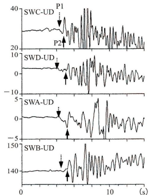
Figure 19. Initial part of displacement waveforms of an explosive earthquake at Suwanosejima volcano. P1 and P2 show the first downward motion (dilatation) and the subsequent upward motion (compression), respectively (after Figure 7-29 of Nishimura and Iguchi, 2011).
