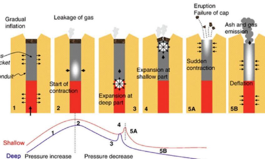
Figure 20. Model of events involved in a volcanic explosion on the bases of geophysical observations at Suwanosejima, Sakurajima, and Semeru volcanoes. Schematic vertical displacement and/or inflation caused by shallow and deep sources are also shown (after Figure 9 of Iguchi et al., 2008).
