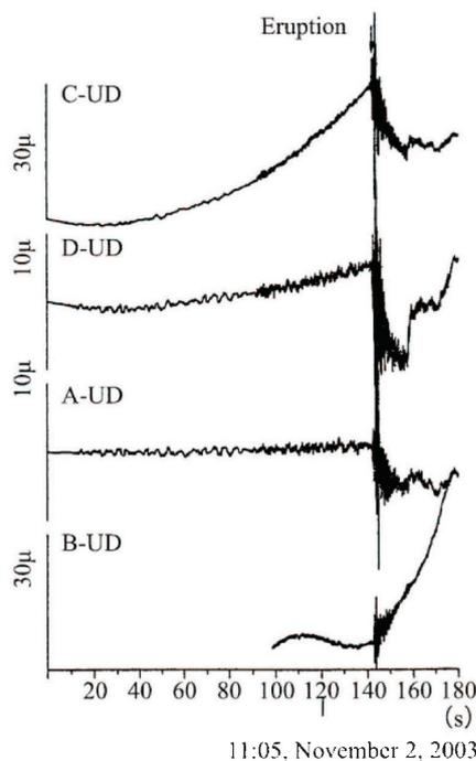
Figure 18. Vertical displacement associated with an explosive eruption at Suwanosejima volcano. The seismograms were recorded by broadband seismometers at four stations around Otake crater (after Figure 4 of Iguchi et al., 2008).
