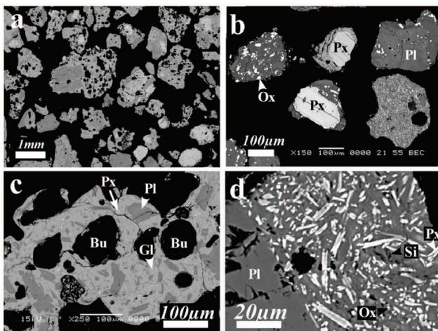
Figure 15. Secondary electron microscope images of ash particles from recent ash falls in Suwanosejima. (a) Representative ash particles from an active period, (b) several particles from a quiescent period, (c) part of a glassy particle with abundant bubbles (C-type), and (d) part of a crystalline particle (D-type). Gl: glass, Bu: bubble, Px: pyroxene, Pl: plagioclase, Ox: oxide mineral, Si: silica mineral.
