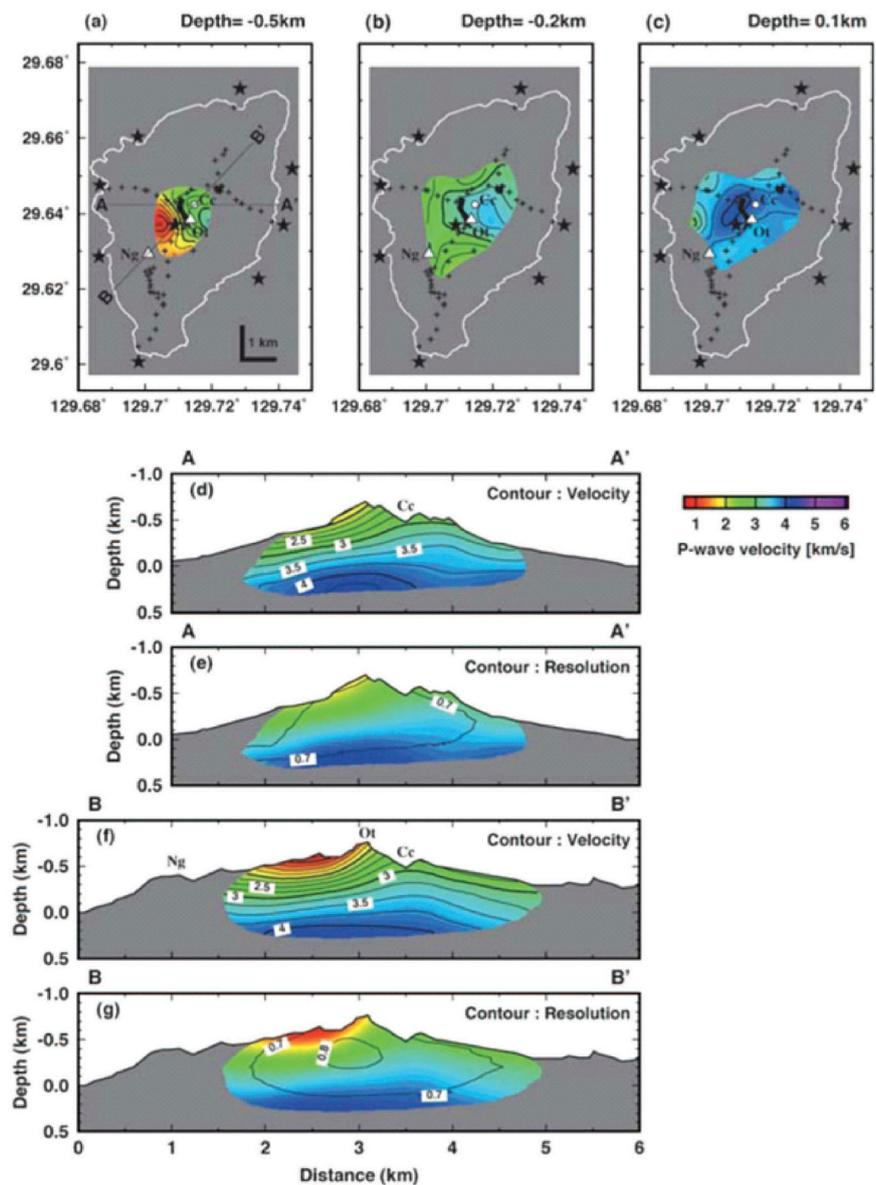
Figure 21. Three-dimensional P-wave velocity model of Suwanosejima volcano. Horizontal and vertical sections are shown with a color index for P velocity. Triangles and a circle denote the summits and an active crater, respectively. Ot: Otake, Ng: Negami-dake, Cc: center of Otake Crater (after Figure 4 of Yakiwara et al., 2010).
